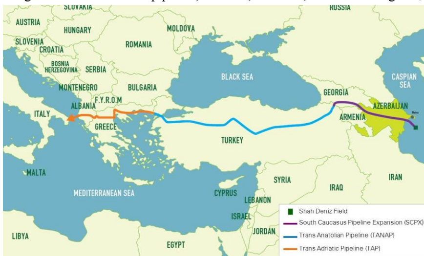
Figure 2: TAP and TANAP pipelines
